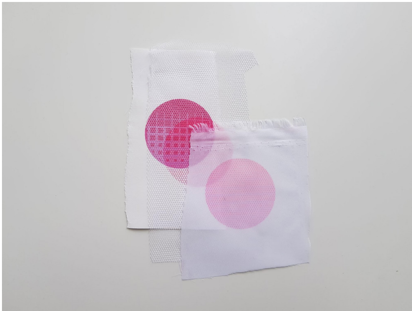
Sublimation print on fabric with a layer of mesh in between
